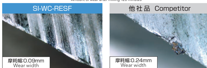
120分加工後の摩耗幅 Amount of wear after milling 120 minutes
